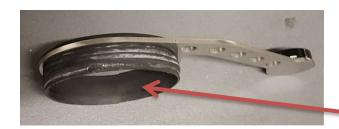
Fit the rubber clamping ring into the holder, smearing a little cream on the inside if necessary, so that it slides better over the watch case.
