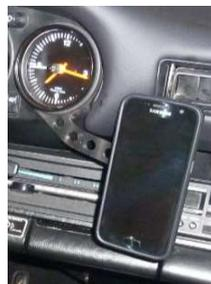
Adjust the position of the holder before pressing in the clock.
